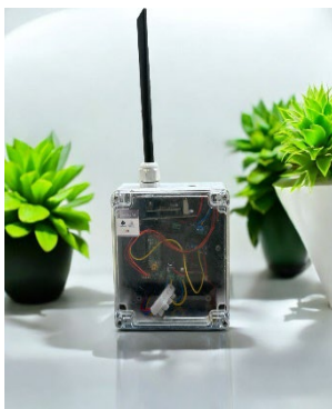
Figure 34: Wi-SUN Router Node
