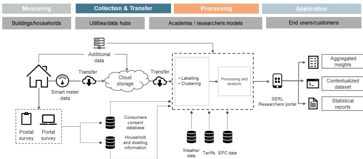
Figure 1: Example data supply chain of smart meter data flow (Source: own illustration based on SERL operating model)
