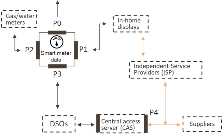
Figure 2: Smart-meter ports and processing, (source: adapted from van Aubel and Pol (2019))
