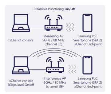
Connect a PC and a smartphone to the main router and measure the speed on the PC when the PC and smartphone are exchanging data as end points. In this case, the smartphone is connected to channel 36 with 80MHz bandwidth in the 5GHz frequency band. On the Sub Router, the PC and Smartphone are connected to each other in the
