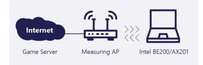
Connect the PC wirelessly (6 GHz) to the router connected to the internet to measure game download speeds.
