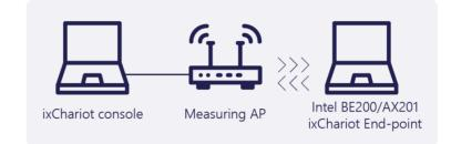
For testing Wi-Fi 7, we used Intel BE200 clients with Wi-Fi 7 AP. For testing Wi-Fi 6, we used Intel AX201 and Wi-Fi 6 AP. The testing computer was wirelessly connected as shown above. The throughput was measured for Wi-Fi 7 and Wi-Fi 6 separately.
