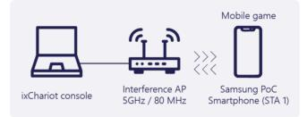
Measure latency in a clean, interference-free environment using only a single smartphone device. This is a control to verify the performance of the QoS Management feature.
