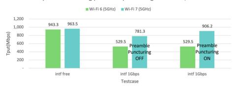
Tput when turning preamble puncturing feature on/off
