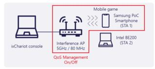
Connect additional PCs to the same router to create an interfering environment, and measure latency while turning on and off the QoS Management feature on your AP and smartphone.
