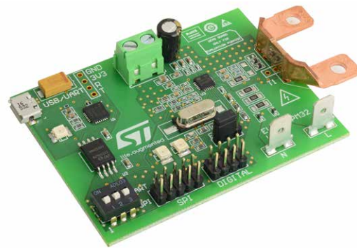
Figure 4: Evaluation board (EVALSTPM32) for a single-phase shunt-based energy meter
