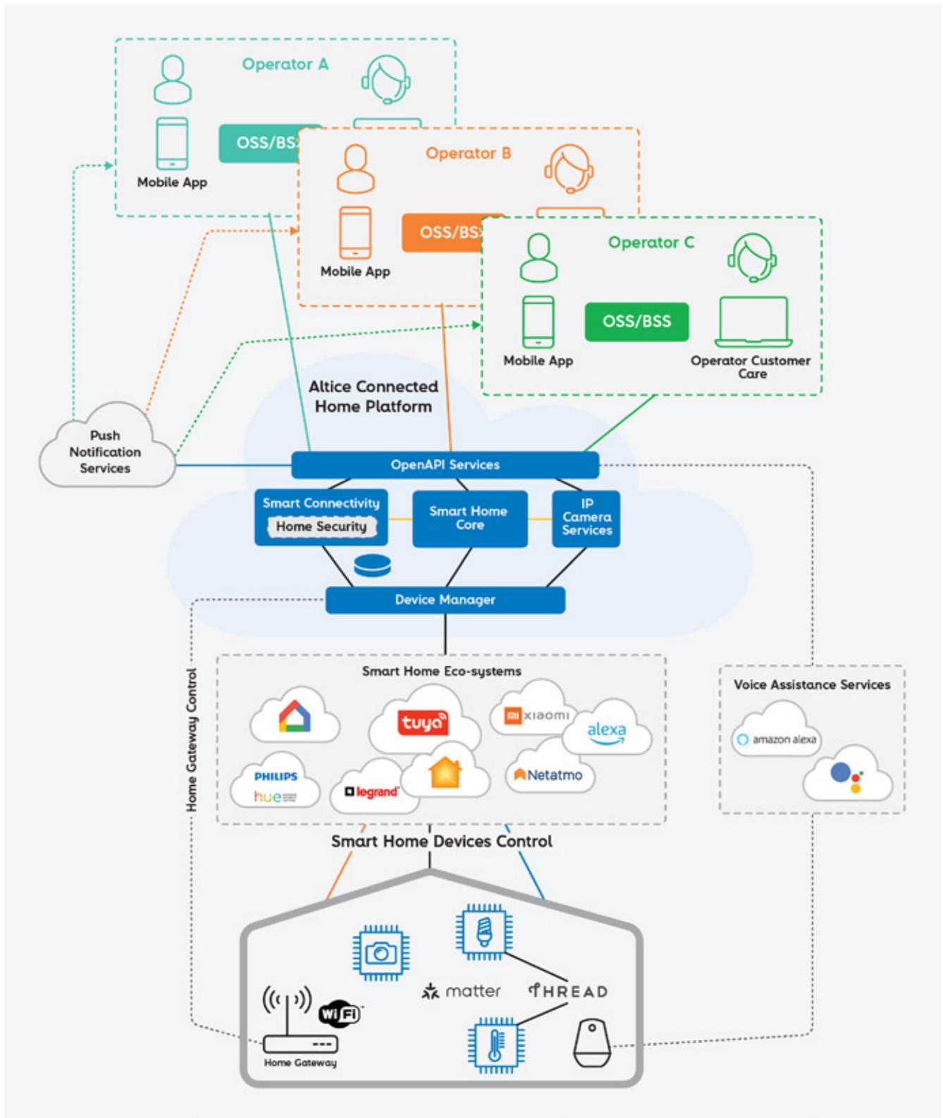
Figure 4 – Altice Home high-level architecture
