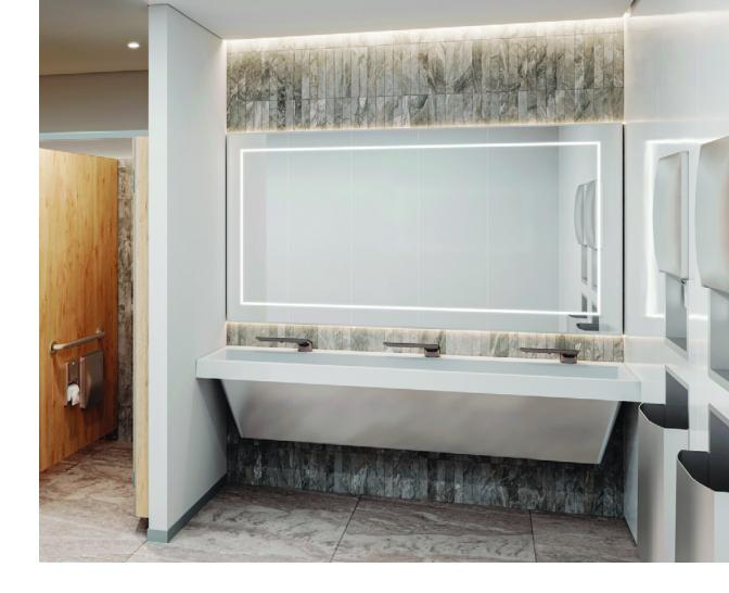
Soap and paper towel dispensers have also been upgraded with maintenance-enhancing technology. Easy-to-read refill indicators predict maintenance and ensure dispensers are well-stocked. A magnetic locking system, which is hidden from sight, also simplifies servicing. Anti-slam operation prevents an open dispenser from banging and damaging walls during refills. An easy-feed towel feature avoids jams and torn paper and eliminates frustration for staff and users alike.
