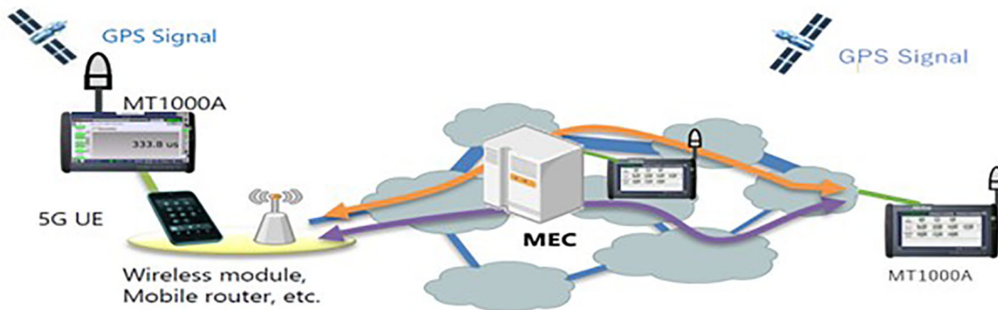
Figure 10: Example of a one-way latency measurement on a MEC.
