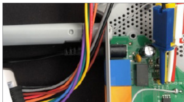
Connecting Logic Analyzer to the device
