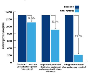
Figure 1. Comprehensive retrofits provide 2.5 to 7 times more energy savings than single measure–based retrofits. Source: Regnier et al. 2018.
