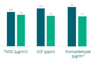
Figure 4. UHealth Fitness & Wellness Center Before and After IAQ Measurements
