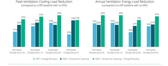
The figure shows that adding high efficiency energy recovery to a VRP-based design can reduce the peak ventilation cooling load by 34-65% and annual ventilation energy load by 40-64%, depending on the climate zone. The chart also shows that adding sorbent air cleaning to an IAQP-based design can reduce peak ventilation cooling load by 60-72% and annual ventilation energy load by 57-61%, respectively, depending on the climate zone.
