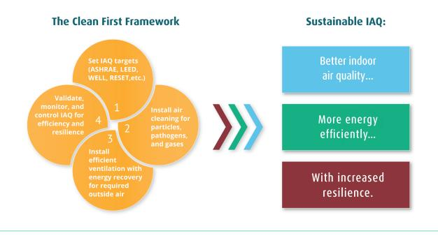
As shown in Figure 2, there are four steps to design and operate buildings using the Clean First framework. For new buildings, it makes sense to start with Step 1 by defining IAQ goals first. For existing buildings, one can start with Step 4 to baseline existing IAQ performance before moving to Step 1.
