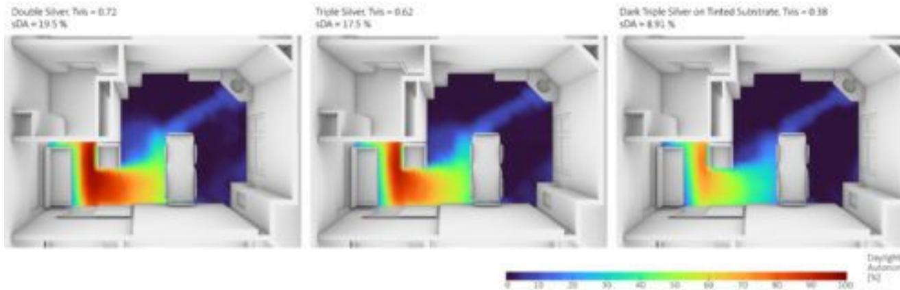
Figure 3: In this example, spatial daylight autonomy is shown for a west facing patient room with decreasing visible light transmittance. The reduced visible light transmittance that accompanies a lower solar heat gain coefficient limits the patient's access to the benefits of daylight. Courtesy: EYP Architecture & Engineering
