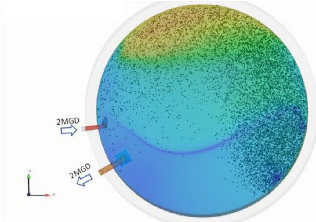
A prime example of this is a CFD study we performed for a client in the central valley region of California, where we used CFD to aid the design of a new pump station intake. Headlosses and flow unevenness were minimized via geometric modifications of the inlet channel and guide walls within the wet well. Pump operational levels were optimized to reduce the potential formation of undesired free surface and subsurface vortices that could threaten the optimum performance of the pump station.
