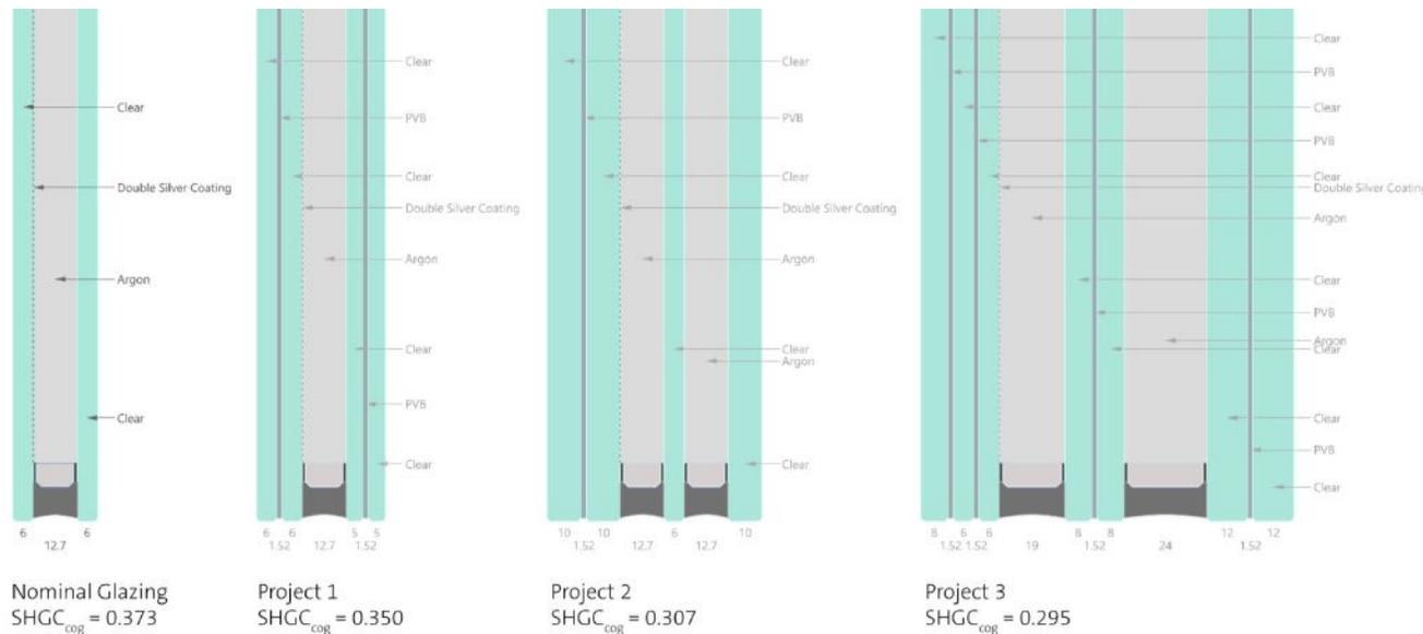
inates, as well as the window unit size and glass-to-frame ratio all additionally modify the total assembly SHGC.
