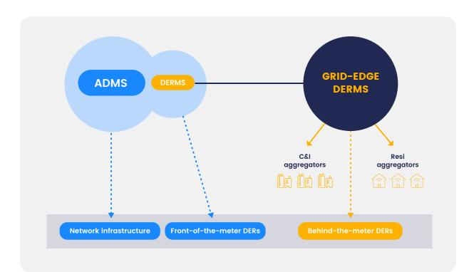
Interaction between the DERMS and the ADMS can take several different forms, depending on the granularity of visibility, control and the nature of information flows between the two systems required to meet utility needs. Network-DER optimization use cases can range from point-in-time, event-based interactions to dynamic, closed-loop intelligent processes. These include:
