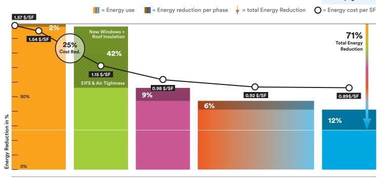
Because the building envelope plays such a critical role in heating demand and overall comfort, additional wall and roof insulation, improvements to airtightness, and the introduction of high performance windows have the greatest impact on energy use, utility cost, and carbon emission reductions.
