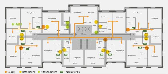
In the proposed scenario the existing ventilation shafts are repurposed, converting the system from exhaust-only to balanced.
