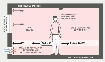
Insulating the exterior and installing high-performance windows ensures that the inside surface temperature of the exterior walls remains warmer throughout winter and, most importantly, closer to the interior air temperature. Research indicates that comfort is significantly compromised when this difference is greater than 7 degrees F. We estimate the existing building suffers from a difference nearly 3x this figure. Graphic credit: Building Energy Exchange
