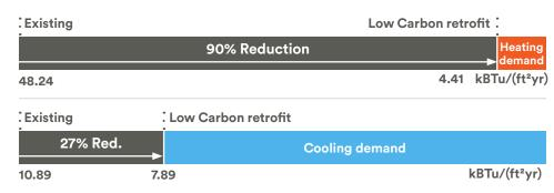
Although a high performance envelope does not reduce the cooling demand nearly as much as the dramatic reductions in heating demand, reduction in cooling demand by 20-30% remains extremely important as that reduction will occur during periods of peak demand for electricity—periods when utility costs and carbon penalties are likely to be highest in the future.
