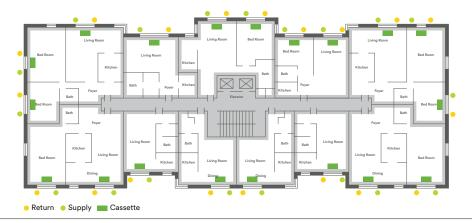
The preferred VRF option in this particular building limits interior construction by placing the new refrigerant lines on the outside of the existing masonry walls and directly accessing the new cassettes over each window. Floor standing interior units are also an option.
