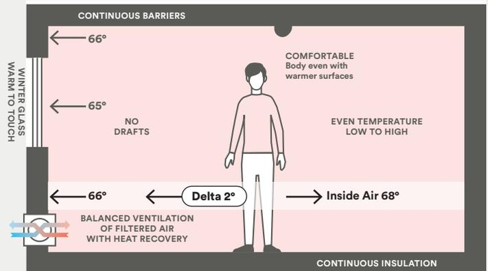
Insulating the exterior and installing high-performance windows ensures that the inside surface temperature of the exterior walls remains warmer throughout winter and, most importantly, closer to the interior air temperature. Research indicates that comfort is significantly compromised when this difference is greater than 7 degrees F. We estimate the existing building suffers from a difference nearly 3x this figure. Graphic credit: Building Energy Exchange
