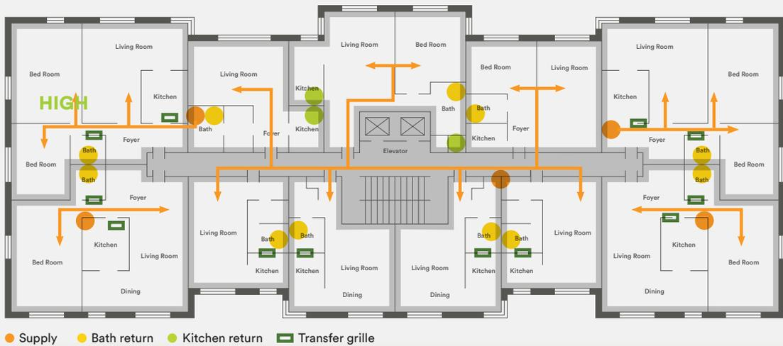
In the proposed scenario the existing ventilation shafts are repurposed, converting the system from exhaust-only to balanced. Rooftop ERV units serve the new supply risers, and transfer grilles allow the refurbished exhaust lines to extract from each room.
