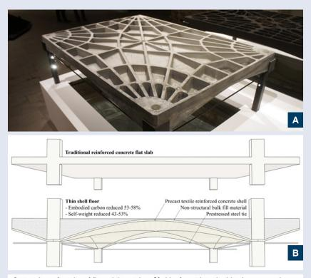
Saving three-fourths of floorslab weight,  $-\frac{1}{3}-\frac{1}{2}$  of a midrise building's structural tons
