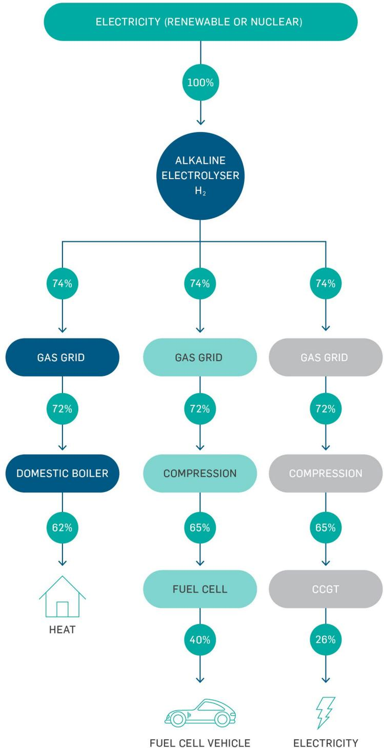
FIGURE 20 HYDROGEN PROCESS EFFICIENCY
