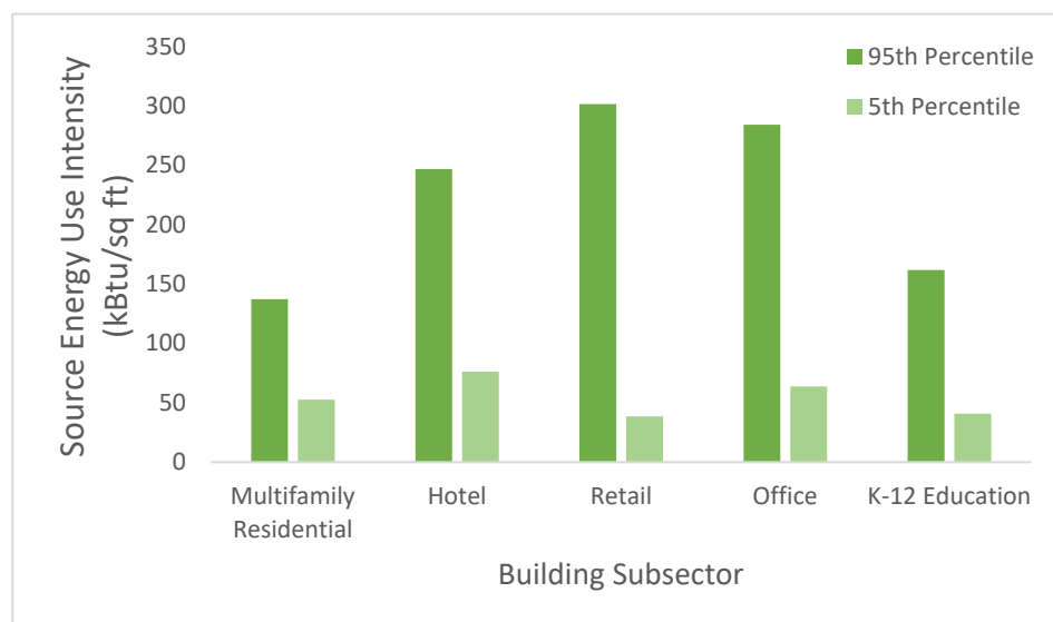
FIGURE 2.3.2 Variation in source energy use intensity (EUI) in five building types. SOURCE: Committee generated using data from Sullivan (2019).
