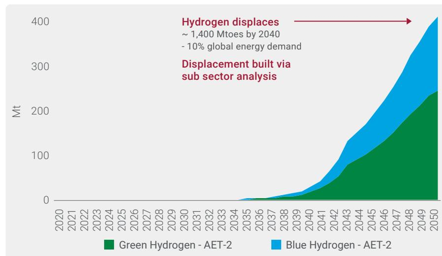
Blue hydrogen comes when SMR hydrogen is paired with CCS while green hydrogen comes from splitting of water molecules using renewable electricity.
