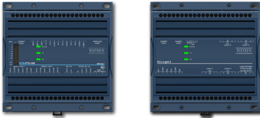
Figure 7: Acuity Distech ECB-PTU series field controller (left) and ECx-Light Expansion Module (right), part of the company’s “Smart Room Control Solution.” Source: https://www.distech-controls.com/en/products/family/room-control-solution
