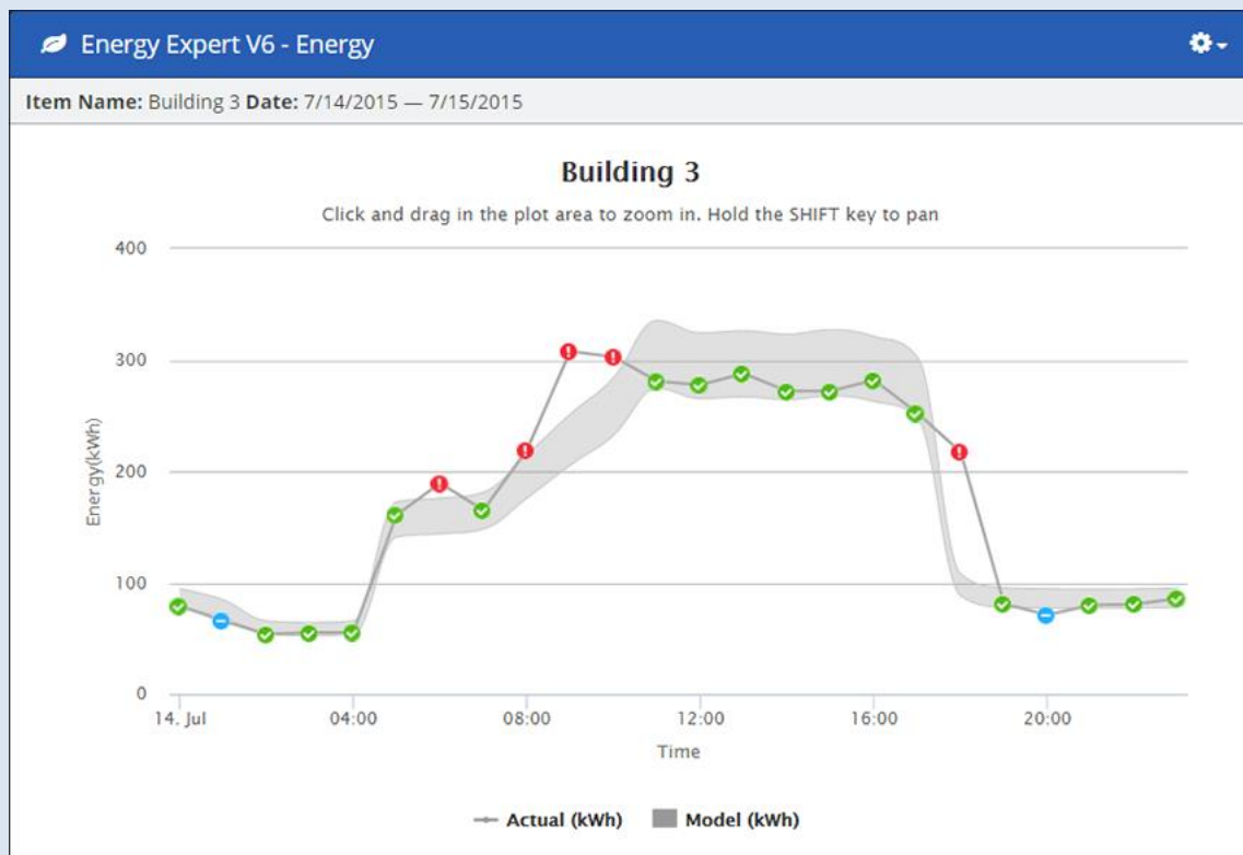
Figure 7. Sample chart from PGE’s Energy Expert data for a single business site
