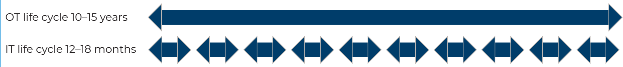
Figure 1. The difference in technology change outs between IT and OT equipment became known as the “life-cycle disparity.”
