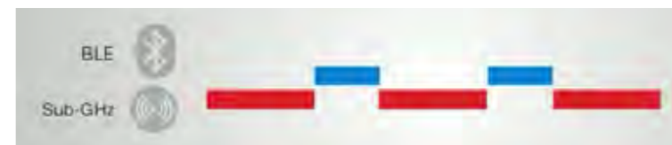
Figure 4: Scheduling BLE and Sub-GHz for multi-protocol applications.
