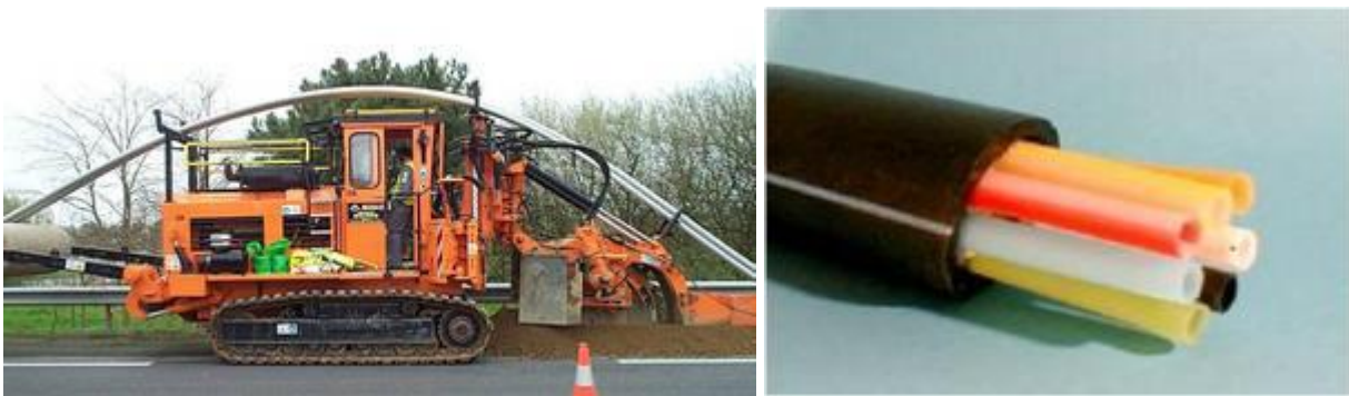
Figure 7: Trenching machine and duct containing multiple subducts
