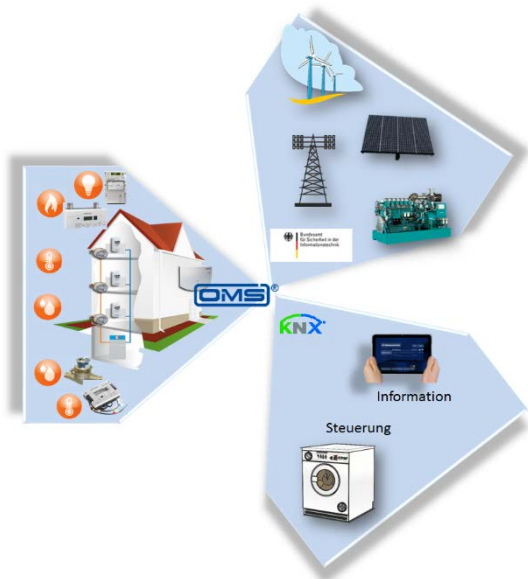
Figure 2: Interplay between metering and sub-metering, home and building automation and energy supply with volatile energy sources.
