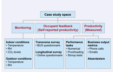
Figure 2 Methodology (temperature, RH and CO<sub>2</sub> level) and outdoor environmental parameters (temperature and RH) were recorded at different locations around the case study offices (6 zones in JCMB, 20 zones in NATS), allowing localised conditions to be monitored and cross-related to individual occupants.
