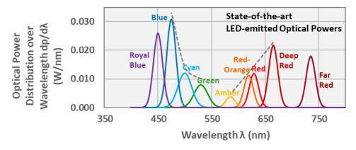
Figure 5-5. Spectral Power Densities of State-of-the-Art Commercial LEDs vs. Wavelength
