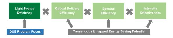
Figure 4-2. Possible Framework for Evaluating Lighting Application Efficiency
