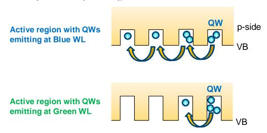
Figure 5-6. Schematic of the LED Quantum Well Valence Band [14]
