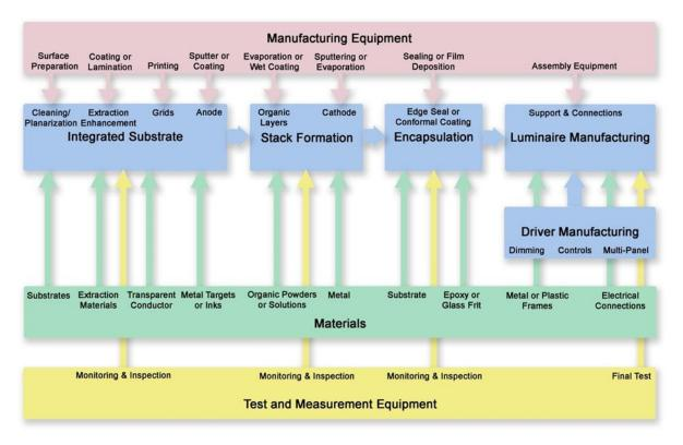
Figure 7-4. OLED-Based SSL Manufacturing Supply Chain
