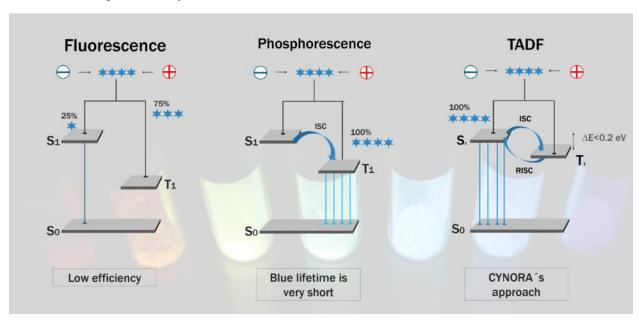
Figure 6-2. Cynora's Illustration of TADF as Compared with Fluorescent and Phosphorescent Approaches [36]
