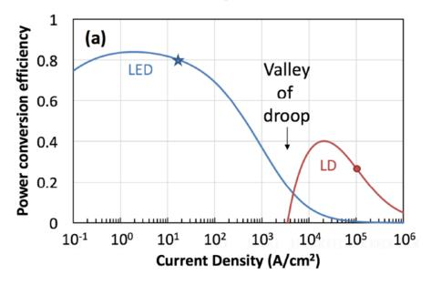
Figure 5-8. PCE Vs. Current Density for a State-of-The-Art LED and LD Emitting at Violet Wavelengths [18]
