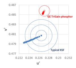
Figure 5-12. Light Loss of Phosphors in LED Packages under High Blue Flux Densities (left) and Color Shift under Stressed Operating Conditions (right) [21]
