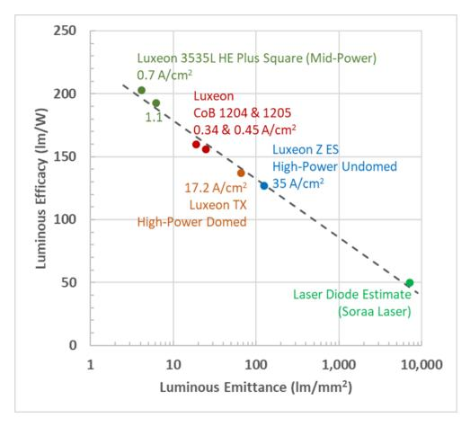
Figure 5-10. Luminous Efficacy vs. Luminous Emittances for State-of-the-Art Commercial White LEDs Note: The dashed line is an empirical fit using the Equation given in the text.
