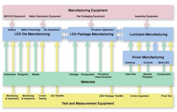
Figure 7-1. LED-Based SSL Manufacturing Supply Chain
