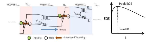
Figure 5-9. Schematic Band Diagram of a Stacked Active Region LED with Tunnel Junctions (left); the External Quantum
