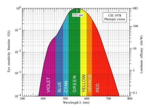
Figure 4-1. Human Eye Sensitivity Function CIE 1978 Photopic Vision Source: LEDs Magazine, Radiometric and Photometric Terms [3]
