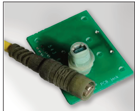
Figure 5: Ruggedized Single-Pair Connector Variant Selected by ISO/IEC for Light and Heavy Industrial Spaces
