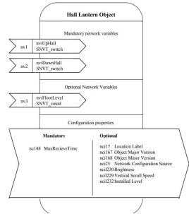
Figure 1: LonMark functional profile of a hall lantern: "UpHall" indicates an uptraveling car; "DownHall" indicates a downtraveling car; "nvi"means an input network variable of the type "SNVT switch".
