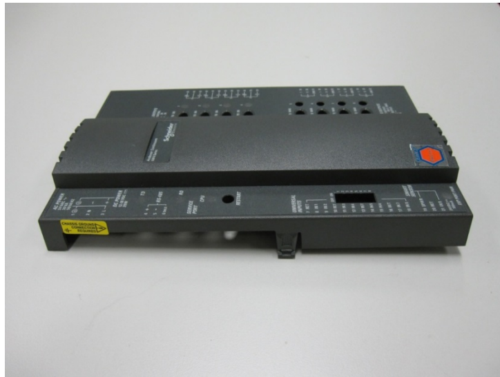
Figure 7.1. Typical AHU Controller Cover
