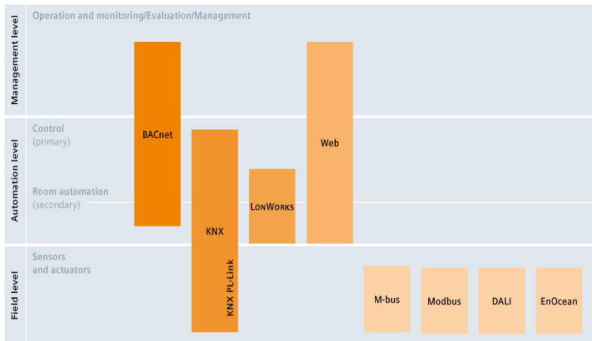
Figure 4.8. BACS Software Architecture (Siemens, 2017)
