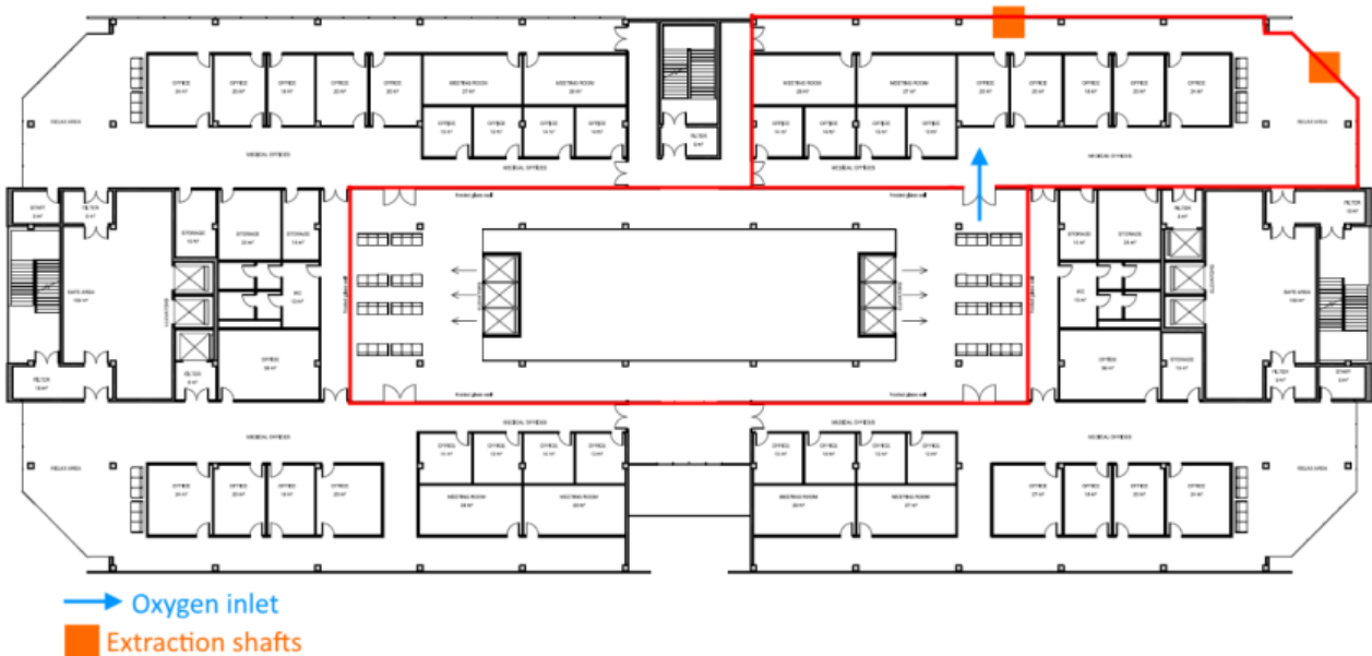
Figure 10 - Fire safety concept on floor 13 th
