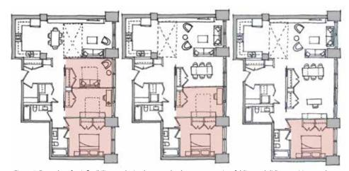
Figure 5. Examples of unit flexibility employing beam-and-column construction, folding and sliding partitions, and sliding pocket doors. Source: City of Toronto, 2017.
