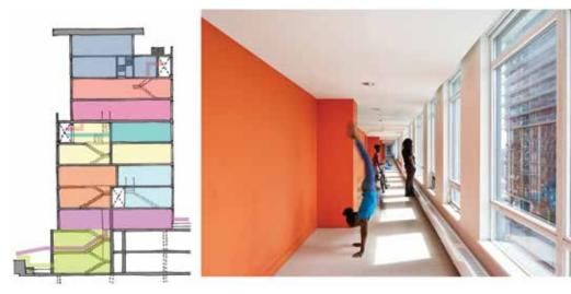
Figure 6. 150 Dan Leckie Way, Toronto – the multi-level "skip-stop" arrangement allows fewer and larger corridors, with finer attention paid to shared spaces. Source: City of Toronto, 2017.
