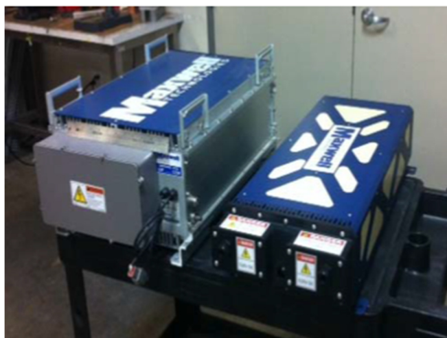
Figure I-2: LICs provide better energy density than conventional supercapacitors. Where energy is important this can reduce the storage device's volume. The unit on the right, developed in the USABC project, is half the size/weight, but twice the power and three times the energy of the standard pack to the left
