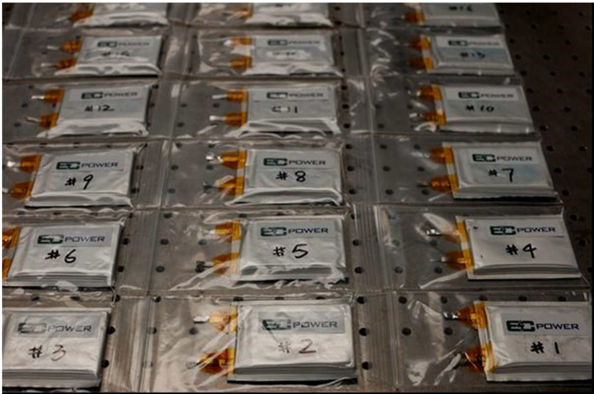
Figure II-71: Picture of eighteen 1 Ah LiP/S pouch cells delivered to INL
