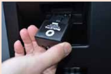
FleetCarma's C2 device that plugs into a vehicle's On Board Diagnostics.
