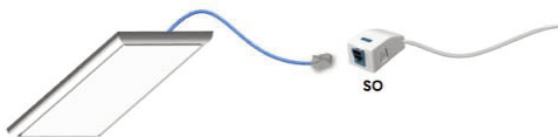
D: 2x4 Fixture Centric - Each 2x4 troffer connects to the structured cabling via a service outlet (SO) or the service connection point (SCP)
