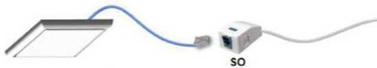
C: 2x2 Fixture Centric - Each 2x2 troffer connects to the structured cabling via a service outlet (SO) or the service connection point (SCP)
