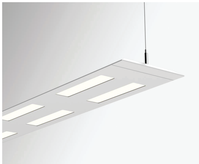
FIGURE 4.2 Acuity Brands Duet SSL™ Technology luminaire. The luminaire combines an OLED that provides diffuse lighting combined with LED uplights that are the primary source of ambient light. SOURCE: Acuity Brands, “Inspiration Through Concepts: Coming Soon... Olessence™ by Peerless® Lighting—Introduced at LIGHTFAIR® International 2016,” http://www.acuitybrands.com/oled/inspiration-through-concepts , accessed August 9, 2016. Courtesy Acuity Brands.
