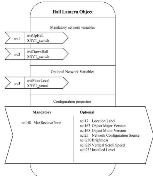
**Figure 1: LonMark functional profile of a hall lantern: “UpHall” indicates an up-traveling car; “DownHall” indicates a down-traveling car; “nvi” means an input network variable of the type “SNVT switch”.**
