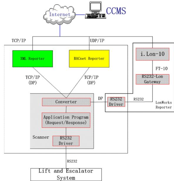
Figure 2: Architecture of ULEG (Universal Lift and Escalator Gateway).
