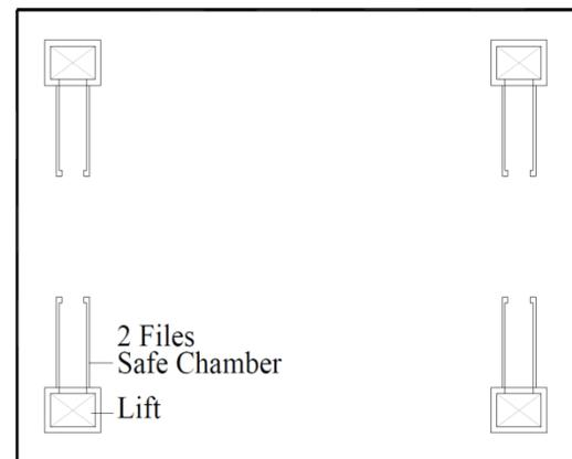
**Figure 4: Refuge floor plan designed with designated elevators at building corners.**
